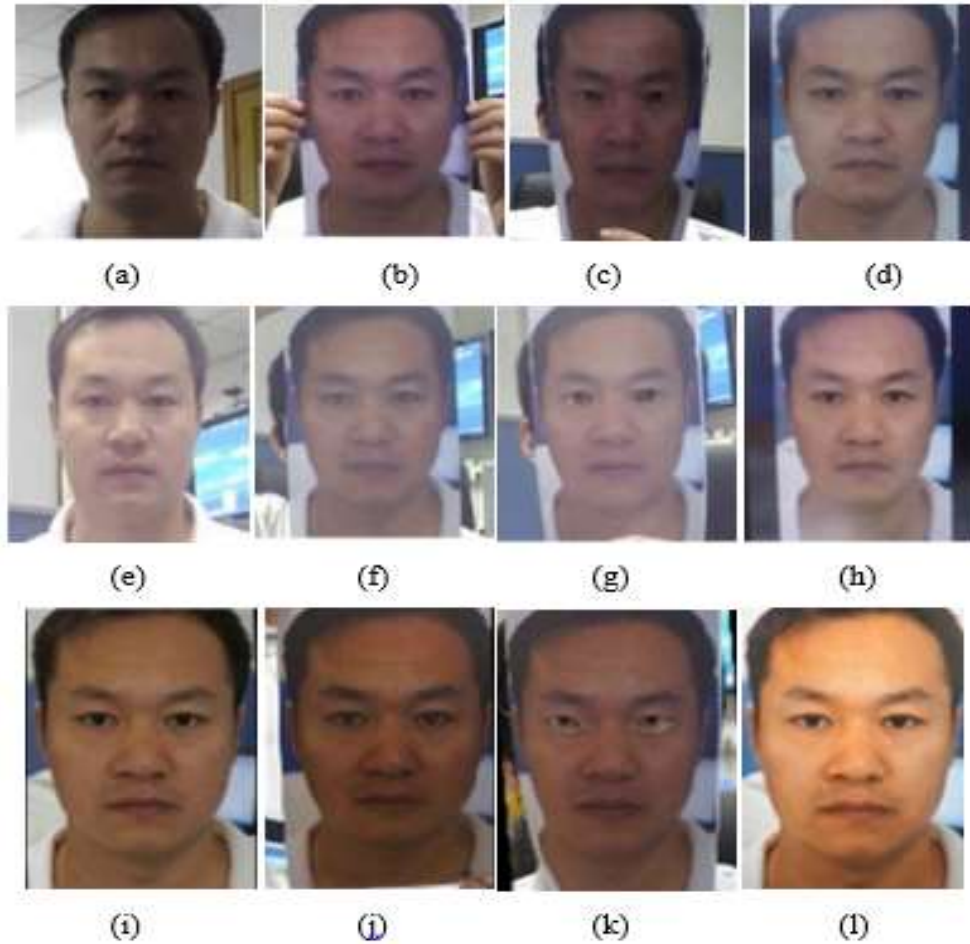
Figure 4. Test CASIA-FA dataset (a) low quality real face image (b) low quality image with warped photo attack (c) low quality image with cut photo attack (d) low quality image with video-replay attack (e) medium quality real face image (f) medium quality image with warped photo attack (g) medium quality image with cut photo attack (h) medium quality image with video-replay attack (i) Low quality real face image (j) Low quality image with warped photo attack (k) Low quality image with cut photo attack (l) Low quality image with video-replay attack
